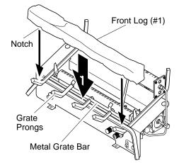
Figure 17 - Installing Front Log (#1)
